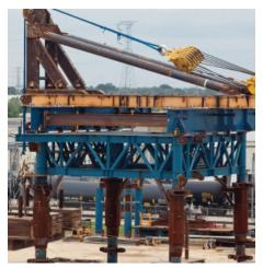
SWOS, and its rope testing partner Versabar, designed a full scale test rig to accurately assess the durability of the custom riser pull-in line as it bends through sheaves during the evolution.
